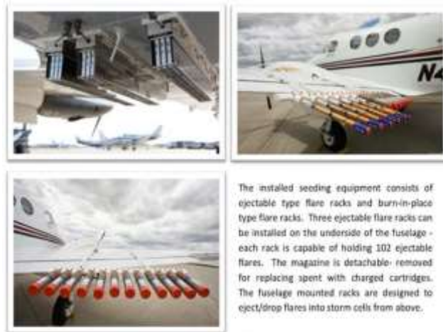
Figure 4. 1. Ejectable Flare Rack and Hygroscopic Flare Rack (Source: Weather Modification Inc. Fargo North Dakota, USA)
