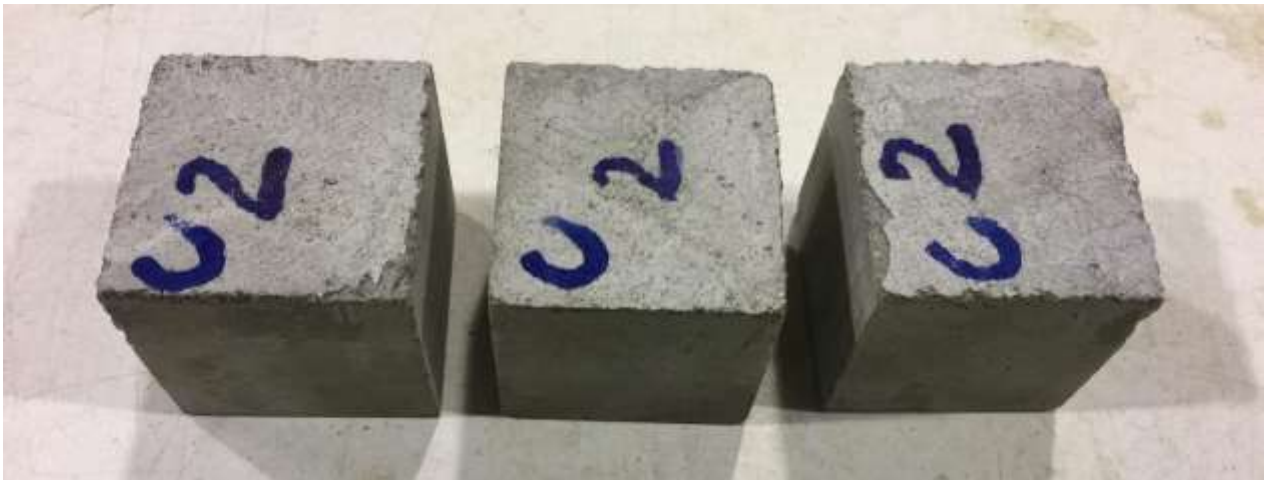
Figure 3. Cubes ready for testing compressive strength of cement-sand grout.
