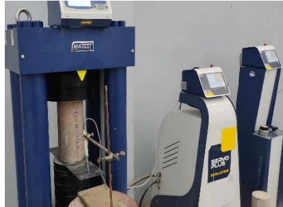
(a) Compression test
