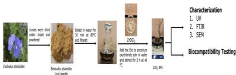
Figure 1 Schematic representation of synthesis and characterization of ZrO 2
