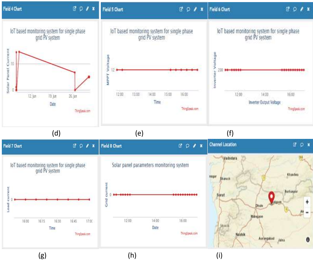
Figure 6. Captured visual data from ThingSpeak platform; (a) Temperature, (b) Solar UV Radiation, (c) Panel voltage, (d) Panel current, (e) MPPT output voltage, (f) Inverter output voltage, (g) Load current, (h) Grid current, (i) channel location.
