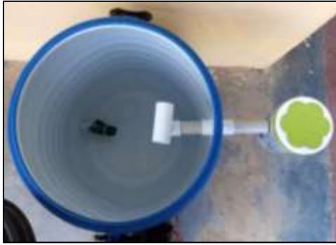
Fig 3: Mini set up for collecting waste and composting using BSF
