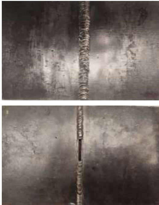
Figure 4 Specimen with induced lack of penetration
