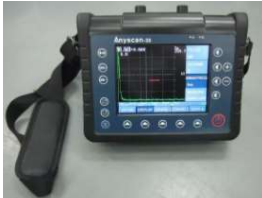
Figure 12 Equipment used in this project. Doppler Anyscan 30.
