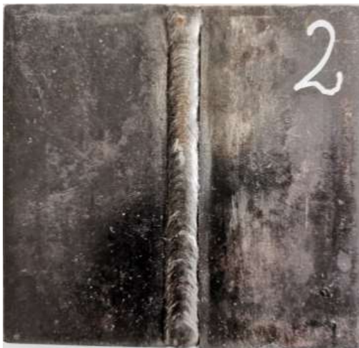
Figure 2 Lack of induced fusion in test tube.
