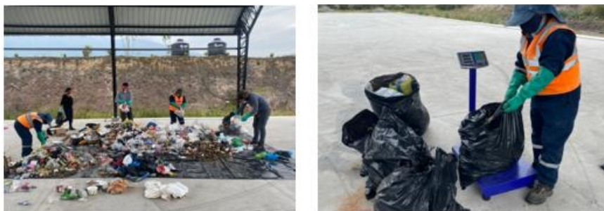
Figure 5. Quartering methodology application at Porlón landfill.
